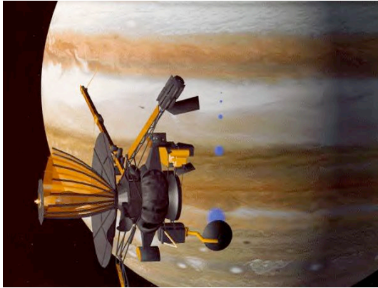
Figure 1. Galileo spacecraft in orbit about Jupiter. One of the two GPHS-RTGs shown at the top. (NASA/JPL)
