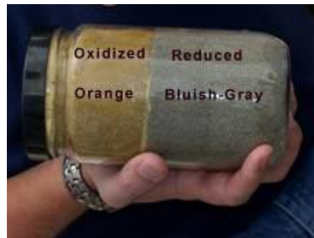
Figure 6a – Typical Oxidized and Reduced Sediments from a Texas Operation.
