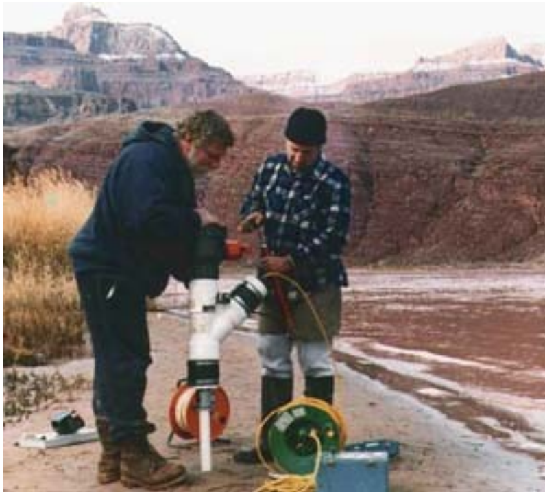
Figure 8 – Typical field slug-testing activities (Northern Arizona University at 2004)
