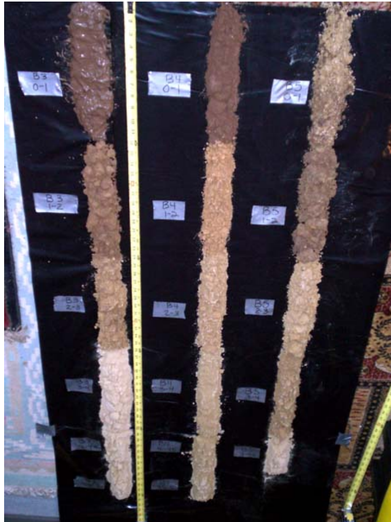
Photo No. 12: Soil profiles of borings B-3, B-4 and B-5. All borings showed clayey silt with some fine sand top soil underlain by weathered fine sandstone starting around 2.5-3 feet below ground surface (bgs). Bedrock, a fine, well-sorted, well cemented, thinly bedded, light gray to tan sandstone was encountered in all borings at approximately 4-4.5 feet bgs.
